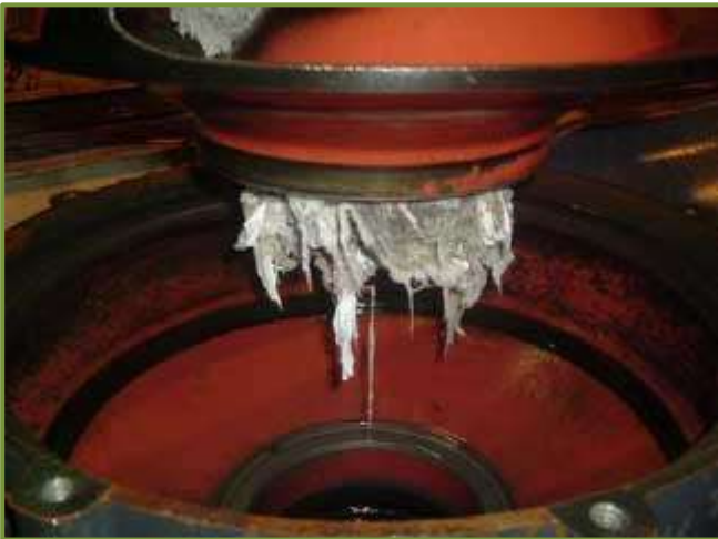
Figures 4.1.1.a & 4.1.1.b – Details the typical extent of a blockage in pump impellers prior to implementing new intelligent control regime.
