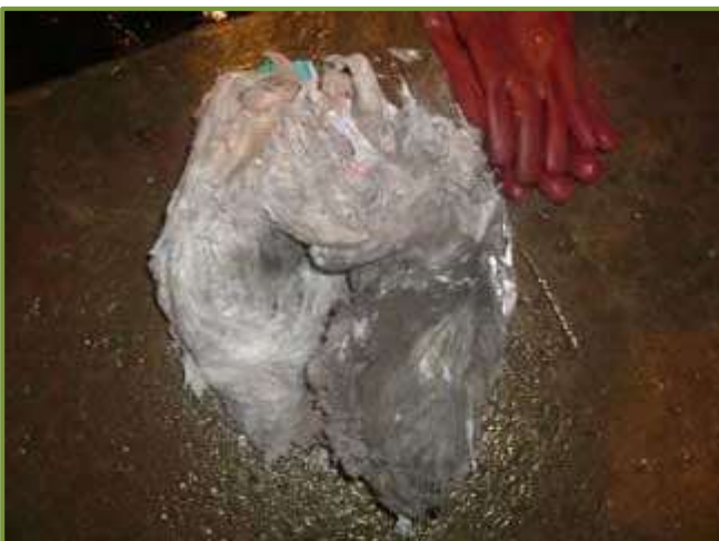
Figure 4.1.1.c & 4.1.1.d – Details the compactness of the blockage material; indicative of compounding over time.
